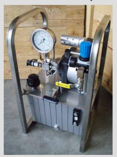
Technofast Air operated hydraulic pumps uses the proven of method a large air piston to drive a smaller hydraulic piston to produce the required pressure.
